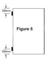
**Figure 5** - The standard practice for fitting rising butt hinges. Assistance should be sought from manufacturer in circumstances where a 3rd hinge is required as a co-axial point must be maintained.
