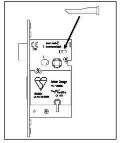
Insert 'T' ensuring rounded profile of 'T' matches the profile of hole in the case.
