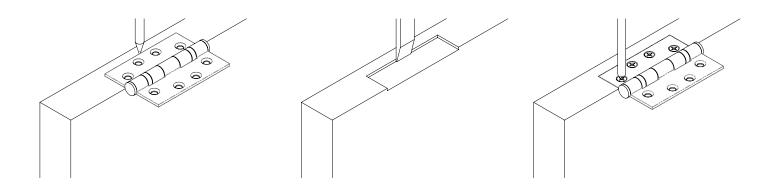
Always refer to manufactures installation instructions for any special requirements. If intumescent pads are being fitted behind the hinge leaf, ensure to increase the mortice depth accordingly. The leaf with the end of knuckle configuration should be fitted to the frame.
