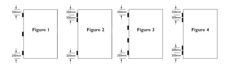
**Figure 1** – The standard practice and most common, providing maximum resistance to "warping", hinges are spaced as shown.
