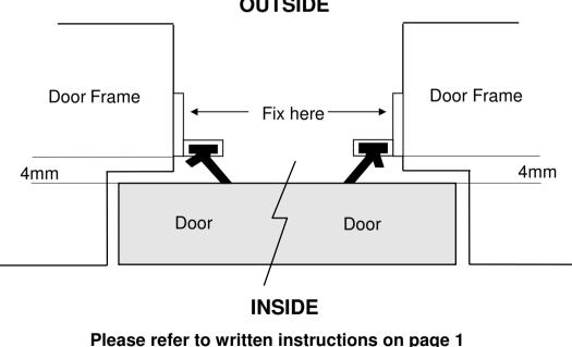
Fig 4a Finished Corner Fig 4 Corners Door frame Door frame
