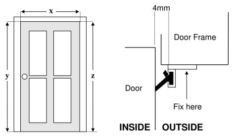
Fig 3 Fitting to door frame and sides (note the different rubber profiles and their relative position)
