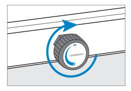
**Step 2.** Turn the gas controls on the appliance clockwise to the OFF position.
