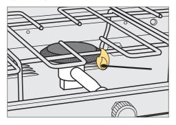
**Step 3.** If the burner does not ignite, turn the gas control in the clockwise direction to the OFF position and allow the residual gas to disperse before attempting to reignite the burner.
