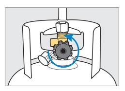
**Step 2.** Take a lit match or lighter and position close to the edge of the burner that is to be ignited, slowly turn the gas control in an anti-clockwise direction approximately ½ of a turn.
