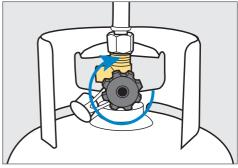
**Step 1.** With the flame still operating, turn the valve on the gas cylinder in the clockwise direction until it is OFF. Allow the flame to burn down then extinguish once all remaining gas in the hose has been used.
