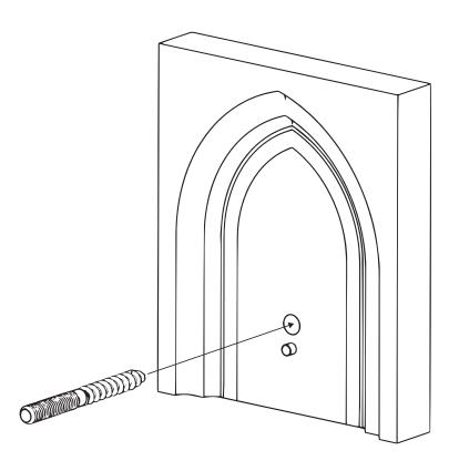
STEP 10: screw hanger bolt in frontplate
