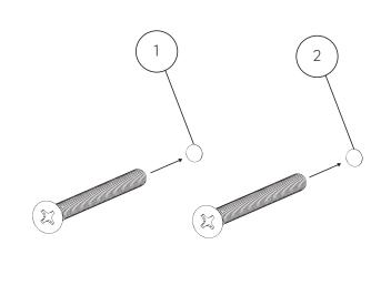
STEP 3: screw M4 screws in wall
