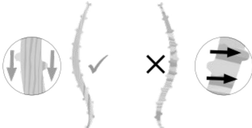
EN - Lay piece face up, so wood grain direction goes up and down the length
