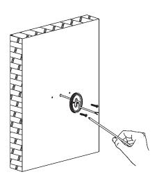
Secure the lower cover of the disc base in the wall with two stainless steel screws to ensure that the power cable passes through the middle of the back base
