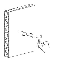
Drill two holes in the wall where the lamp will be installed and insert the wall plug into each hole with a hammer
