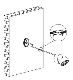
Connect the wire to the lamp to be installed with a waterproof connector
