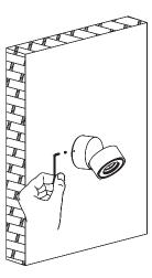
After fixing the lamp and base, lock it with two headless screws
