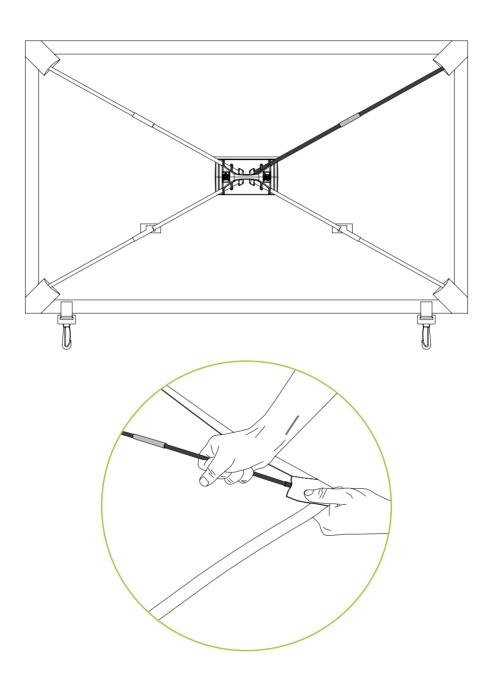
Pull the corner of the backboard away from the center and pre-bend the fibreglass rod to create enough space to insert the rod into the corner pocket.
