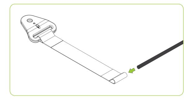
Thread 1x fibreglass rod assembly through 1x L**ow Mount Pole Strap (7)** as shown.
