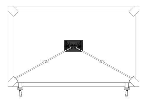
Insert each end of the fibreglass rods into the **High Mount Cross Bracket (4)** as shown.
