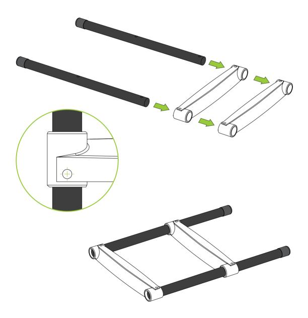
Take the **Ladder Hooks (16)** and insert into the top of the **Ladder Poles (15)**, hooks facing down and ensuring the drilled holes align with the holes in the **Ladder Poles (15)**.
