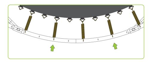
Attach another **Spring (4)** in the middle of each new spacing until all the frame attachment points are connected to the **Jump Mat (5)** D-Rings as shown.
