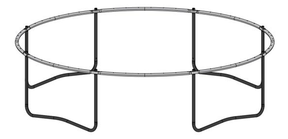
Repeat steps 1-5 until all the **Top Rail (1)** and **W-Foot (3)** components are assembled making the complete circular frame of the trampoline.
