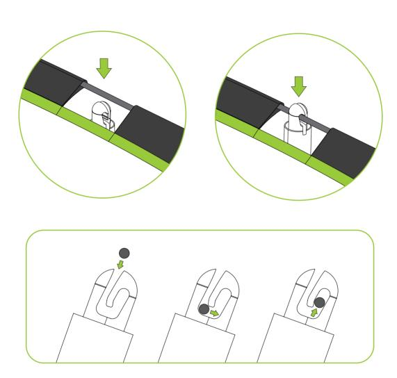
Ensure the fibreglass ring is pushed down, and then
