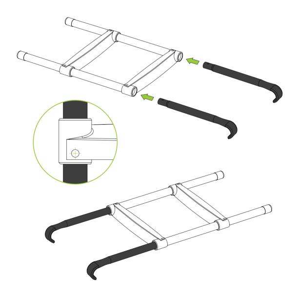
Using the supplied **Screwdriver (17)**, take the **40mm Bolts (18)** and screw them through the four holes until tight to fully assemble the ladder.
