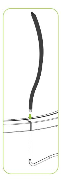
Take the net pole assembly and feed the bottom through the hole in the **Spring Pad (8)** and into the **Leg Pole (2)**. Ensure the button clip is aligned and clicks into place. Pull the **Spring Pad (8)** back over the edge of the frame.
