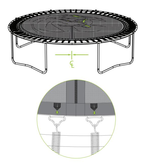
Important: Align the net zip exactly in the middle between two legs. Count out the springs from left to right of each leg and locate the two middle springs. Locate and align the two safety net attachment rings either side of the zip and align them with these springs and the corresponding D-Rings on the Jump Mat.
