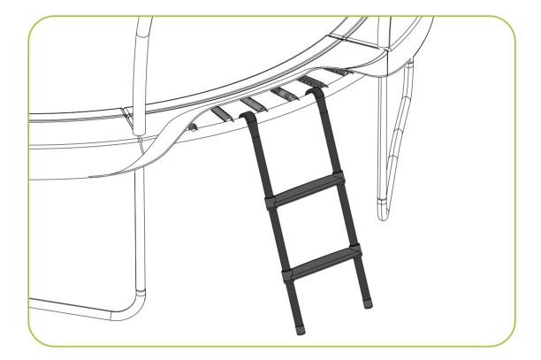
Take the fully assembled ladder and place it over the top rail on the trampoline.
