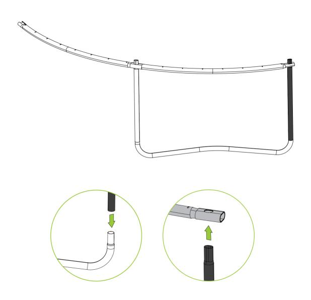
Make sure the springattachment holes are facing upwards.
