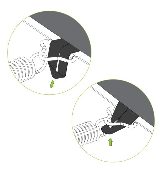
Starting at the net zip, take a fabric hook from the base of the **Safety Net (8)** and thread it through the **Jump Mat (5)** D-Ring and over the attached hook. Work your way around the trampoline, repeating this process until all the fabric hooks are attached.
