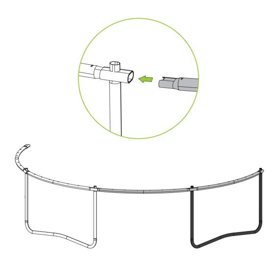
Repeat steps 1-4 and then attach the assemblies together by bringing the **Top Rails (1)** together as pictured.
