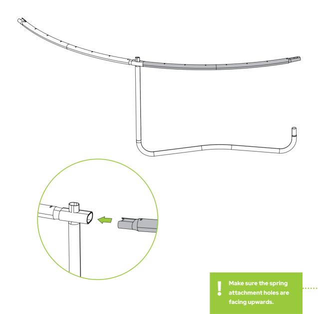
Place 1x Leg Pole (2) on to the W-Foot (3) and insert through the Top Rail (1).
