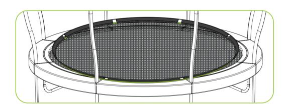
Take the fibreglass ring at the top of the **Safety Net (7)** and push it down through the plastic hooks on the top of the **Safety Net Poles (9)**. Repeat until the fibreglass ring is secured in all the **Safety Net Poles (9)**.
