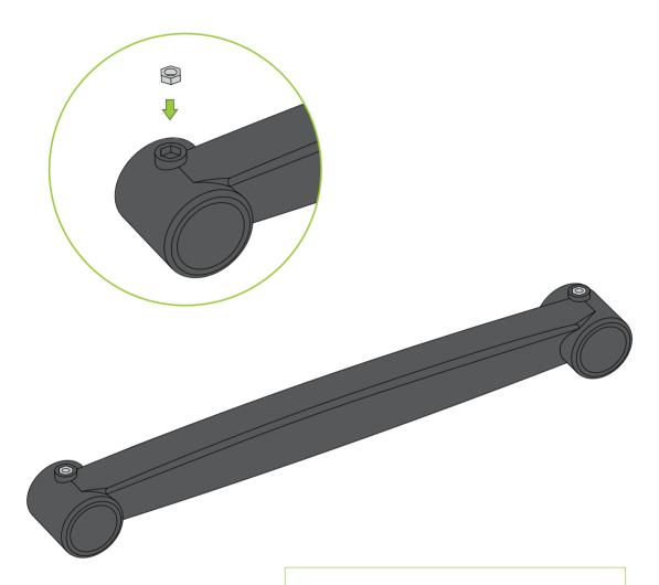
Take out the **Ladder Steps (13)** and the **Ladder Nuts (14)**. Push the four **Ladder Nuts (14)** into the hexagon recesses on the back of the two steps.
