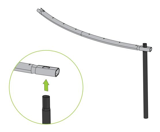
Make sure the top rail is curving away from you and the spring holes are facing upwards.
