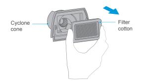
Clean the dust cup: Flap the filter cotton (remember that not to flap in reverse direction).
