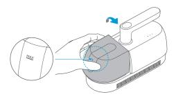
Above the trash can, take out the filter components and clean the dust.
