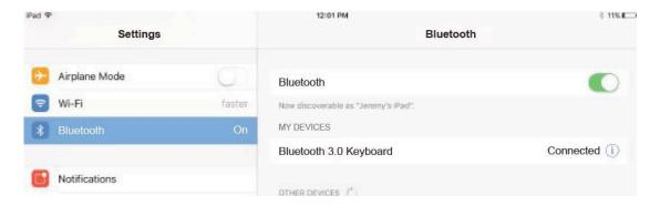
After your successful first-time pairing, your iPad will automatically remember the keyboard. To connect again, please turn On Bluetooth on your iPad, and the keyboard. The device should automatically connect. If it does not connect, please tap it in the My Devices list to connect.
