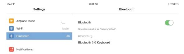
3.Tap "Bluetooth 3.0 Keyboard" - the pairing process is complete after "Connected" appears (see photo below.)
