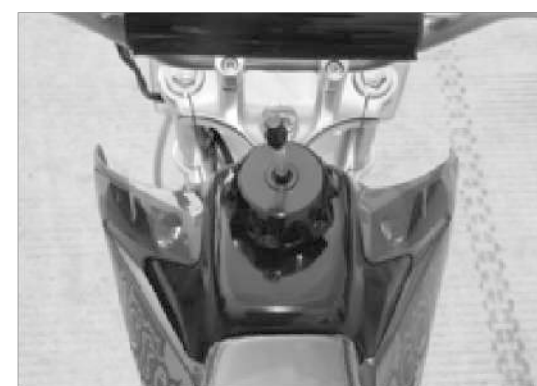
5. The fuel Cover: Note: the fuel Cover mouth ventilation can not plug.
