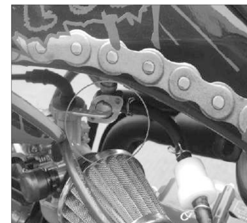
6. The fuel valve: the fuel valve in the fuel filter will supply fuel from the fuel tank to the carburator. Fuel valve has two locations.
