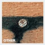
Although corrosion of fasteners can eventually impact structural integrity, unsightly staining, streaking and discoloration are often more common and immediate concerns. Given the high costs of labor, lumber and other building materials, paying a little more for top quality stainless steel fasteners (compared to plain or galvanized steel) is a good step toward preventing corrosion and protecting your investment.
