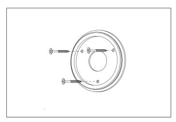
Fix the wall plate to the wall by using wall mounting plugs and screws suitable to your wall type.
