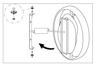
${f 3.}$  Place the lamp over the crossbar and fix it with the screws.
