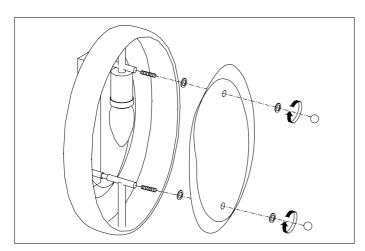
5. Attach the glass to the lamp with the screws supplied.
