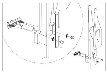
4. Place the lamp over the crossbar and fix it securely with the nuts.
