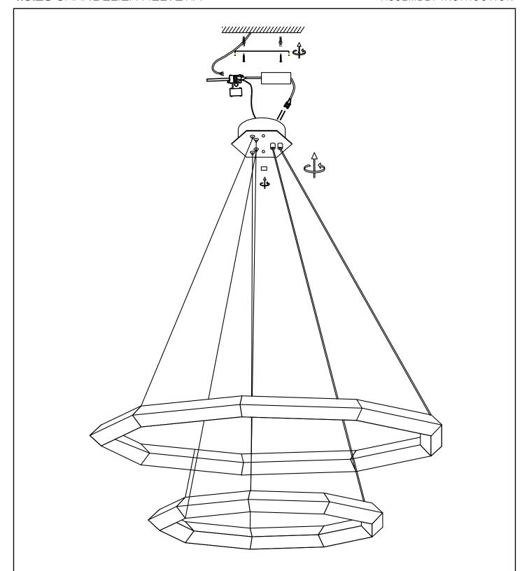
Fix the crossbar to the ceiling by using mounting plugs and screws suitable to your ceiling type.
