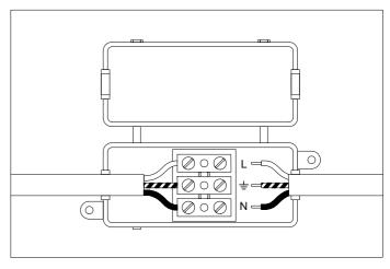
2. Connect the 3 wires according to their colours. Brown is the live wire (L), blue is the neutral wire (N), green/yellow is the earth wire  $(\frac{\bot}{-})$ .
