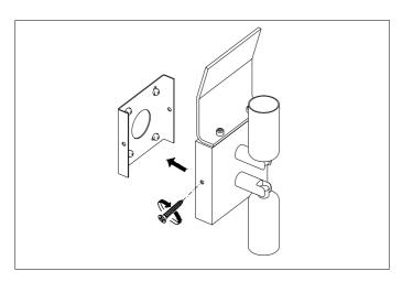
3. Place the lamp over the crossbar and fix it securely with the screws supplied.
