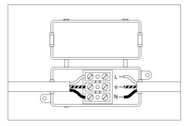
$\label{eq:connect} \begin{array}{l} \textbf{2. Connect the 3 wires according to their colours. Brown is the live wire (L), blue is the neutral wire (N), green/yellow is the earth wire (<math display="inline">\underline{+}). \end{array}$
