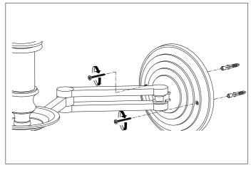
2. Place the lamp over the plugs and fix the lamp to the wall by using suitable screws for your wall.
