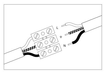
1. Connect the 3 wires according to their colours. Brown is the live wire (L), blue is the neutral wire (N), green/yellow is the earth wire ( $\frac{L}{w}$ ).
