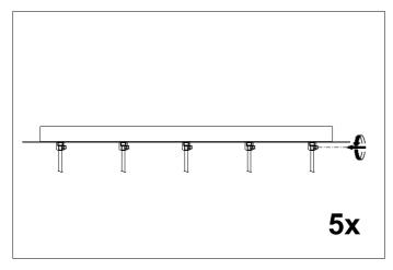
3. Put the wire through until the lamp is at your desired height and fix it with the plastic nuts.
