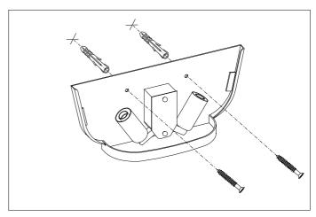
${\bf 2.}\,{\sf Fix}$  the lamp to the wall by using wall mounting plugs suitable to your wall type.
