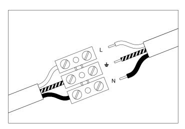
1. Connect the 3 wires according to their colours. Brown is the live wire (L), blue is the neutral wire (N), green/yellow is the earth wire ( $\frac{1}{4\pi}$ ).
