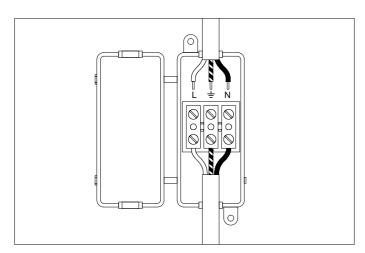
3. Connect the 3 wires according to their colours. Brown is the live wire (L), blue is the neutral wire (N), green/yellow is the earth wire ( $\pm$ ).
