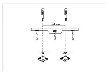
2. Fix the ceiling plate to the ceiling using mounting plugs and screws suitable to your ceiling type.
