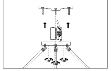
Place the ceiling canopy flush against the ceiling and fix it securely with the 3 nuts supplied. Tighten the nuts with tools, not just by hand.
