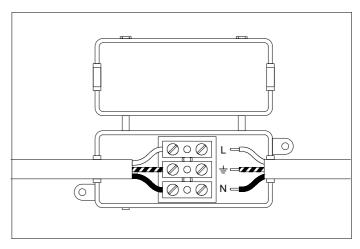
**4.** Connect the 3 wires according to their colours. Brown is the live wire (L), blue is the neutral wire (N), green/yellow is the earth wire  $(\frac{1}{2})$ .
