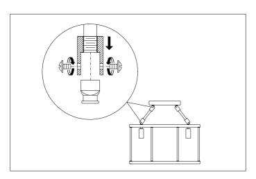
1. Fix the pipes with the screws supplied.
