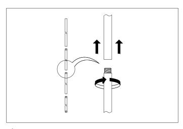
1. Determine the desired height of the lamp and use either one, two or three of the pipes supplied. Thread the wires through the pipe.
