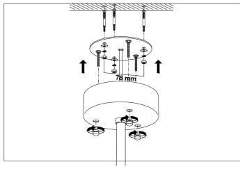
**3.** Fix the bolts to the ceiling. Then fix the ceiling plate to ceiling with screws.
