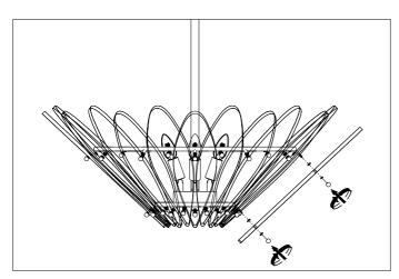
5. Place the glass and fix it with the nuts supplied.
