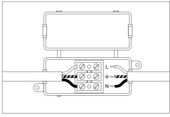
2. Connect the 3 wires according to their colours. Brown is the live wire (L), blue is the neutral wire (N), green/yellow is the earth wire ( $\frac{\bot}{-}$ ).
