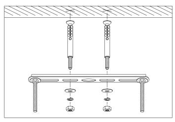
1. Fix the ceiling bracket to the ceiling by using mounting plugs and screws suitable for your ceiling type.
