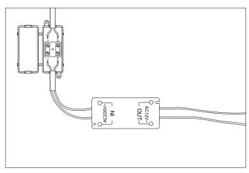
Place or hold the lamp in an elevated position in such a way that the wires can freely reach the ceiling junction box. Connect the 2 power wires. Brown is the live wire, blue is the neutral wire.
