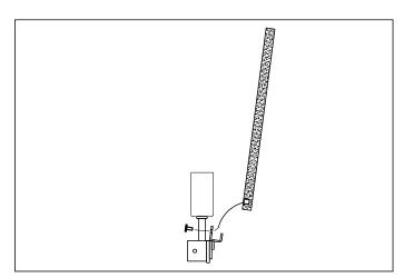
3. Place the alabaster plate in the holder and fix it with the screw.
