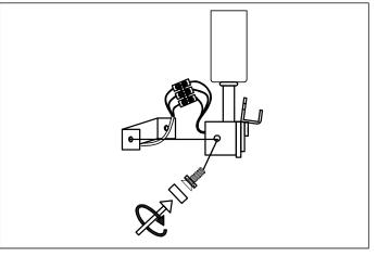
2. Connect the 3 wires according to their colours. Brown is the live wire, blue is the neutral wire, green/yellow is the earth wire. Place the lamp over the crossbar and fix it with the screws on the side.
