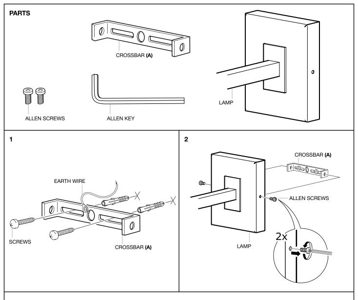
Turn off the electricity supply at the main circuit panel before installing.
