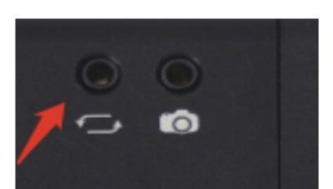
Plug the sync cable for Slider
