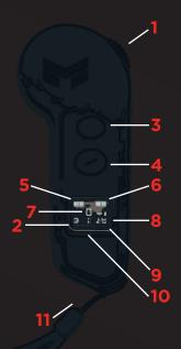
4\* Forward/Reverse – Double Tap 2\* to cycle between Forward and Reverse. Direction will be represented by arrow on right.
