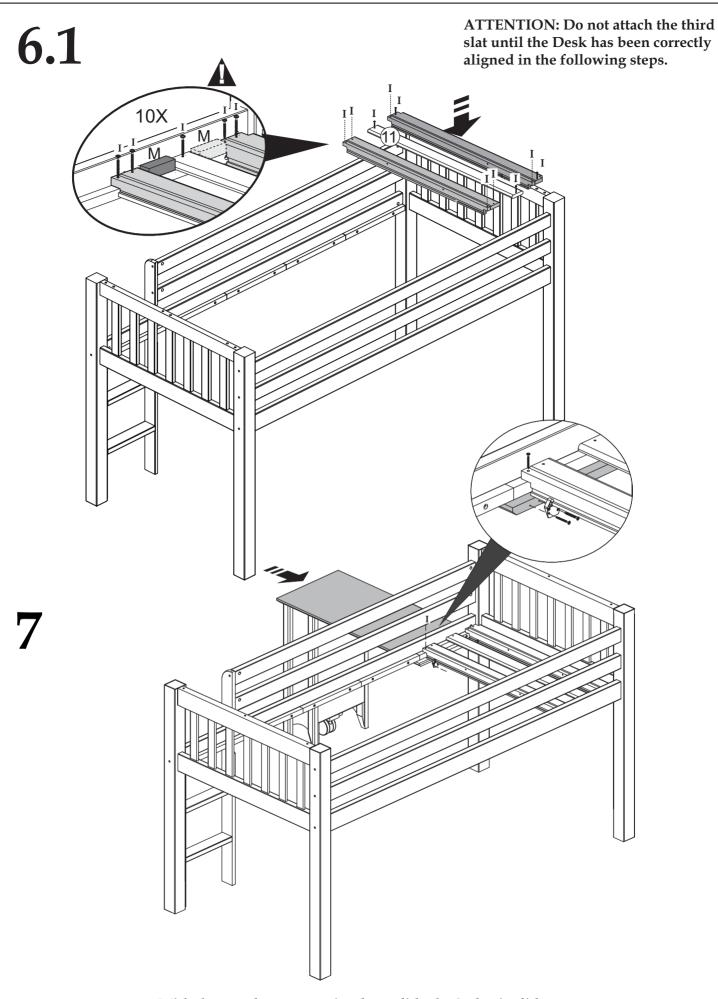
With the wooden runners in place, slide the 2 plastic sliders to the front of the bunk and attach to the edge of the desk using 4 screws. At this point fix the front side of the third slat using another screw, as detailed above.
