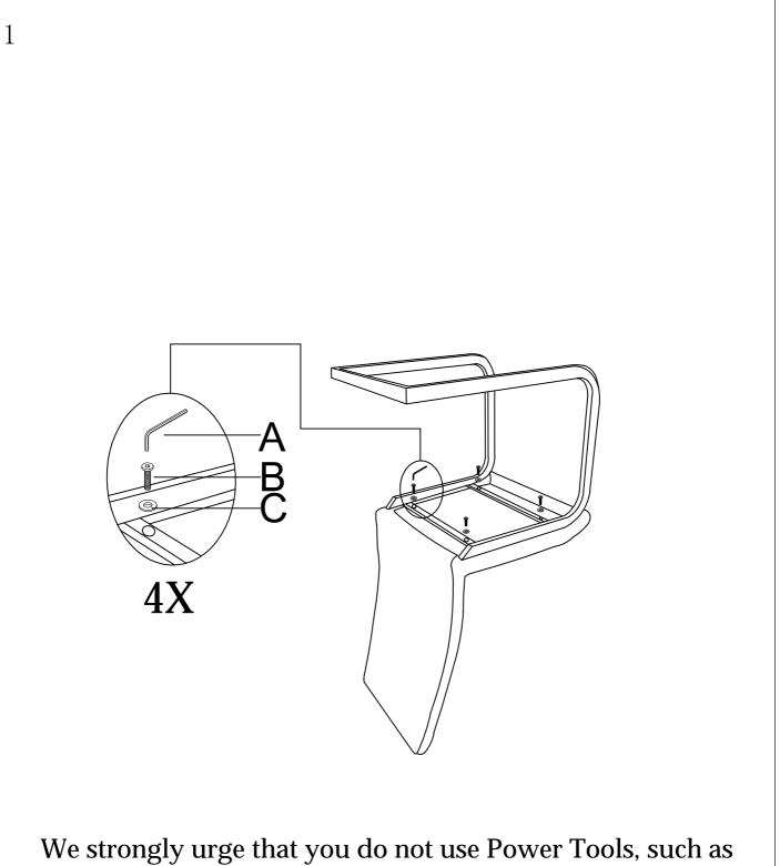
We strongly urge that you do not use Power Tools, such as drills or electric screwdrivers during this assembly as this could cause irreparable damage to your product and will invalidate the warranty.
