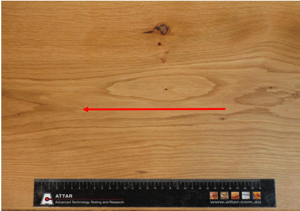
Figure 1: Evolution Hardwax Oil applied to engineered timber flooring Arrow indicates direction of testing
