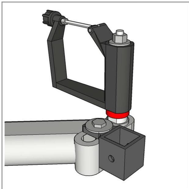
Grab the Female Pontoon Brackets to make sure they are snug. The bolt flange should fit flush with the top of the rigger and the receiver tube should fit flush with the vertical, bow-side surface of the rigger.
