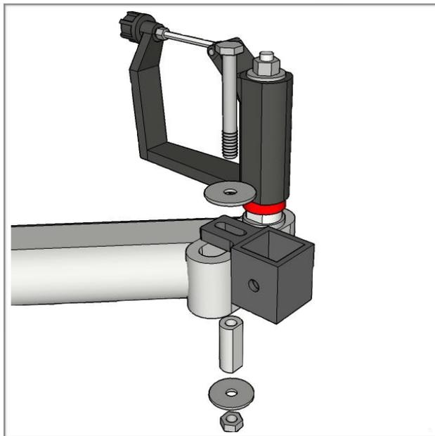
Bolt the Female Pontoon Brackets to your rigger according to the diagram on the right. Insert the aluminum spacer into the Euro slot of your rigger first, followed by the fender washers, bolt and locking nut. If you should have any trouble inserting the aluminum spacer into the slot of your rigger, rotate the spacer until the machined flat on the spacer allows it to fit. Use two 7/16" wrenches to tighten the bolt and locking nut until the bottom fender washer becomes slightly concave.
