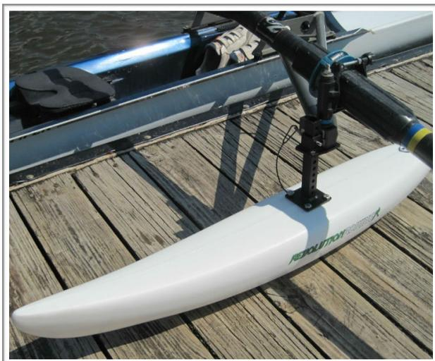
Do not leave your dockside Stabilizer Pontoon attached while at the dock as damage to your pontoon, brackets and rigging may occur. Attach your dockside Stabilizer Pontoon only after you have launched.
