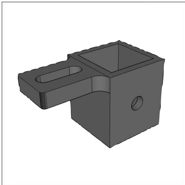
Your Female Pontoon Brackets consist of two parts: the bolt flange and the receiver tube. The bolt flange has an oval slot that is used to bolt the bracket to your rigger, while the receiver tube has a long square tube to receive the Male Pontoon Brackets.
