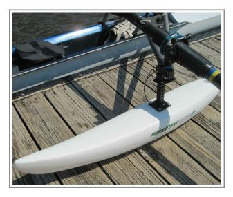
Do not leave your dockside Stabilizer Pontoon attached while at the dock as damage to your pontoon, brackets and rigging may occur. Attach your dockside Stabilizer Pontoon only after you have launched.
