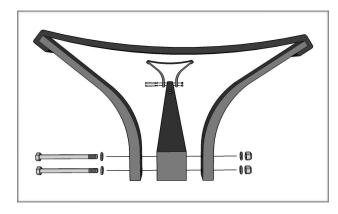
Use the (4) 1/4 inch X 4 1/2 inch bolts, (8) 1/4 inch flat washers and (4) 1/4 inch nylock nuts to attach the (2) "V" cradles to the assembled main rail. The cradles attach to the ends of the main rail that have (2) holes. Attach the bottom bolts first, and the top bolts second. Tighten all nuts and bolts with your 7/16" wrenches <u>only</u> as tight as you can get with your pinky fingers.
