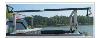
Do not transport your boat cockpit up. Our single scull roof racks were designed to transport boats by the decks of the boat, which are much flatter than the hull of the boat. Transporting your boat cockpit up will result in unnecessary rocking and movement during travel. Transporting cockpit up will also potentially allow for the collection of rainwater.
