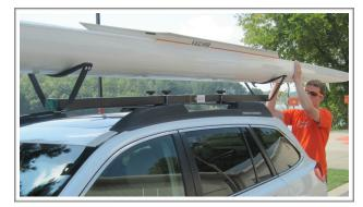
Slide the hull of your boat forward onto the Single Scull Car Rack until the cockpit of your boat is centered between the front and rear cradles. For taller vehicles, you may have to position a step ladder near the bumper of your vehicle to assist with loading.
