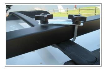
Tighten the lobed knobs on the U-bolts so that the plates bend over the rail of the Single Scull Car Rack. U-bolts should be attached such that they are at opposing angles. Once tightened, grab the rail of your single scull rack and shake. The entire car should move such that you hear your gas tank sloshing. **Warning! Re-check the tightness of the U-bolts frequently during travel.**
