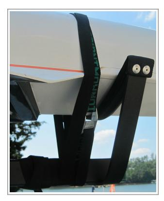
If you have excess webbing from the straps, make one more wrap around the hull of the boat and then wrap the remaining webbing around the main rail of the single scull rack. Tie off the last few inches so that the webbing does not flap in the wind during travel. If you prefer to make the webbing extremely secure, you can use a couple wraps of electrical tape to secure the loose end of the strap. **Warning! Do not wrap excess**
