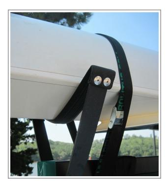
Use (2) boat straps to secure your boat to your single scull rack. Straps should be located directly to the inside of the front and rear cradles so that they wrap around the boat and the main rail on the single scull rack. Straps should be pulled tight enough so that they are snug and so that the boat pulls down into the cradles. **Warning! DO NOT over tighten the**
