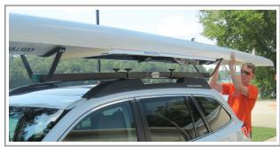
Rotate your boat from cockpit up to cockpit down. You may need to lift the stern of the boat so that the cockpit gunnels do not hit the rail of the Single Scull Car Rack while rotating. **Warning! Always transport your** scull cockpit down.
