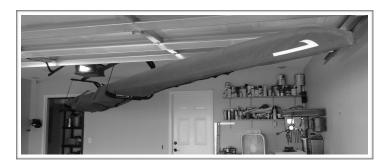
5. Rotate the handle on the winch slowly to lift your scull about a foot off of the ground. Double check that the brake on the winch works correctly by rotating the handle backwards and lowering your scull back to the ground. If the brake works, go ahead and rotate the handle on your winch until your boat is fully lifted.
