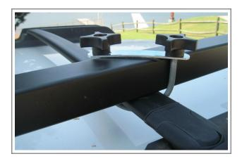
Tighten the lobed knobs on the U-bolts so that the plates bend over the rail of the double scull rack. U-bolts should be attached at opposing angles. Once tightened, grab the rail of your double scull rack and shake. You should move the entire car such that you hear your gas tank sloshing.
