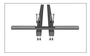
Use the (8) 3 1/2 inch X 1/4 inch bolts, (16) 1/4 inch flat washers and (8) 1/4 inch nylock nuts to attach the (2) Padded Crossbars to the assembled main rails as shown. The crossbars attach to the ends of the main rails with (2) holes. Tighten all nuts and bolts with your 7/16" wrenches only as tight as you can get with your pinky fingers.
