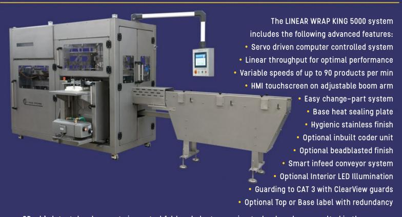
CPack's latest developments in control fold and pleat wrapping technology have resulted in the LINEAR WRAP KING 5000. Utilising advanced computer control, combined with servo technology, our system provides unparalleled flexibility, adaptability and performance. Ideal for wrapping cheese, pies, cakes, burgers and other round products at speeds of up to 90 products per minute.
