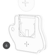
Pull the CR2032 up out of the battery contact.
