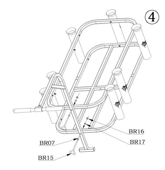
4. Connect handle stand to frame assembly. Tighten nuts snugly.
