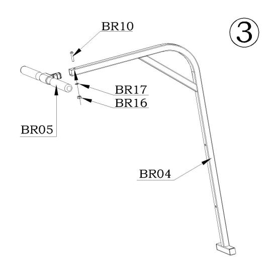
3. Insert handle into handle stand. Secure using bolt with washer and lock nut. Tighten nut snugly. Do not over tighten.
