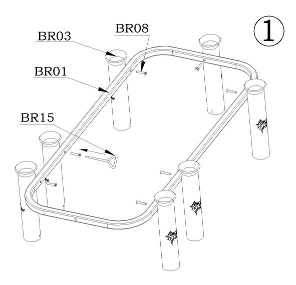
1. Attach rod holders to upper frame assembly. Tighten bolts snugly. Do not over tighten.
