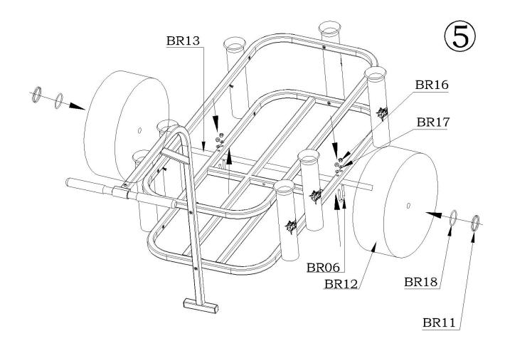
5. Attach axle to lower frame assembly with U-bolts. Tighten nuts snugly. Do not over tighten. Attach wheels to axle using washer and split ring.
