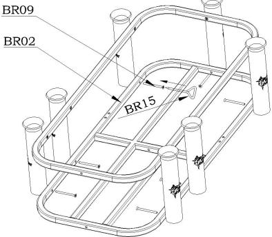
2. Attach lower frame assembly to bottom of rod holders. Tighten bolts snugly. Do not over tighten.
