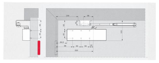
With this fixing method, the max closing force is approx. 20 Nm (for doors up to 950mm) Parallel-arm bracket (accessory) necessary
