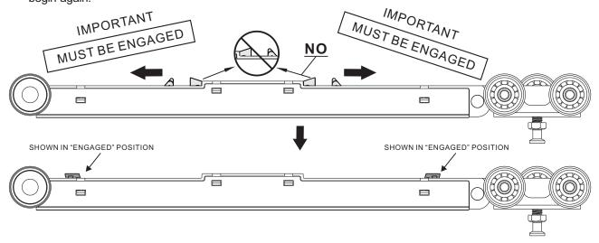
5 Insert Soft Close Hanger into Track.(Idle wheels first)
