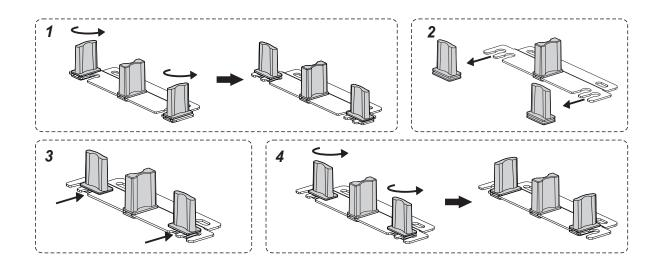
ONLY push the back actuator/trigger 80 mm to left as shown in following figure. NOTE: The front actuator/trigger don't need to move position.
