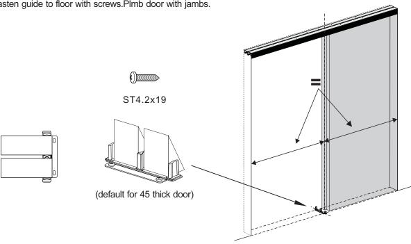
Floor guide installation instruction for 35mm thick wood door:
