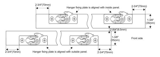
**9** Hang Doors. Start with front door first. Slide pivot pin of hanger into socket and click the tab in place. Check for smooth travel. Repeat with rear door.
