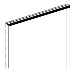
Mount Hanger Plates to Door: Fasten door plates to top of door,2-3/4"(70mm) from each edge.
