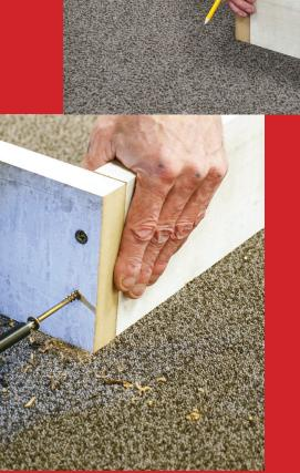
Pre drill the lintel twice at each end from the top and countersink these holes to allow it to accept the screws that will secure it to the top of the legs.
