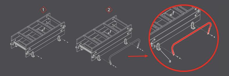
**GB** For ladders where the spring is mounted on to the bracket "a", the spring has to be disengaged before mounting the handrail. Disengaging the spring may only take place when the ladder is in a closed position. Remember to mount the spring again after fitting the handrail.
