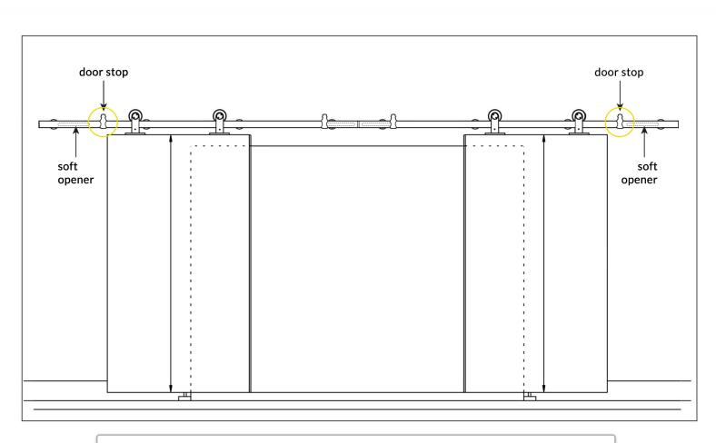
Installing all soft openers is advisable, just keep in mind that the soft openers will not function when opening the doors. Use the door stops provided to prevent the doors from extending beyond the floor guides and becoming disengaged when open.
