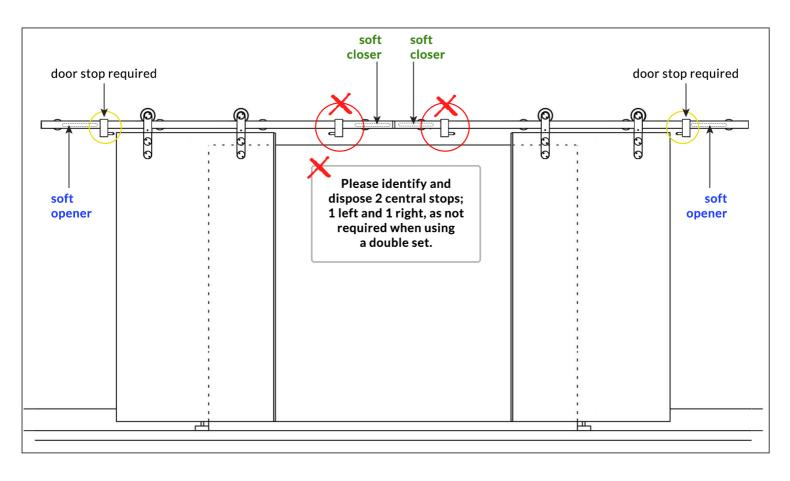
For optimal performance, it's advisable to install both soft closers and soft openers on double doors. The soft closer will facilitate smooth door closure. However, please note that the soft openers will not function when the doors are fully open.
