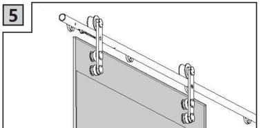
Attach the face fix track hangers to the door and then hang the rollers to the track.
