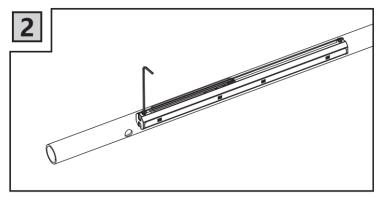
Take of the end cap from the track and one wall fixing bracket, put the soft close/soft opener inside and fix it with screws supplied (see installation video).
