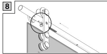
Push the door to the soft close/soft open to make it triggered by the actuator.
