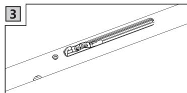
Set and fix the trigger with the screws supplied, re-fix the wall fixing bracket and track end cap.
