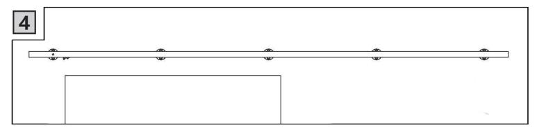
Set up and fix the track to the wall or any strong frame (see track assembly instruction in the track box), track must be properly levelled.
