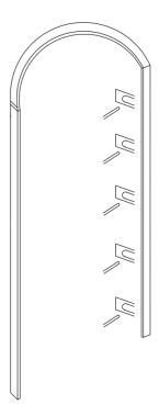
• Following the dimensions drill through the frame on the opposite side at the top of the frame (see below). Secure with frame fixing and horseshoe packers.
