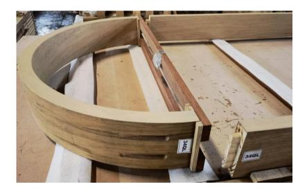
With the vertical frame jambs lined up with the curved frame top, remove the two
