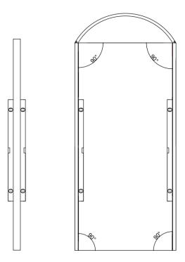
• The positioning of the frame fixings must be planned in advance and we recommend positioning them so they'll be hidden by the loose stop once it's in place. A maximum of 550mm is recommended between fixings. See frame fixing locations below.
